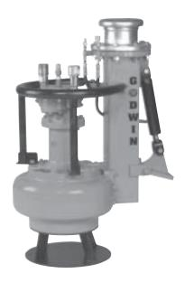
The Heidra 150VSG is a versatile, 6" (150mm) hydraulic submersible pump capable of passing large solids up to 5" (125mm), stringy materials and slurries. A remotelyoperated slurry gate allows the pump to act as a mixer, ideal for pumping thick, viscous, solids-laden sludges, such as those found in WWTP digesters, environmental clean-ups and API separators at refineries.
